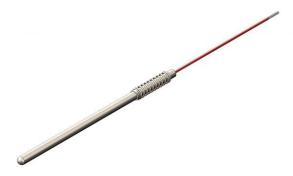
Designed for applications where a General Purpose Head and a thermowell are required. The spring-loaded action of this RTD ensures proper contact with the tip of the thermowell for maximum heat transfer.
