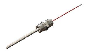
Designed for applications where a spring-loaded threaded male fitting is required for mounting. It is intended to be used with a thermowell and to be compatible with any head that will accept a 1/2" NPT instrument thread. The spring-loading action of this RTD ensures proper contact with the tip of the thermowell for maximum heat transfer.
