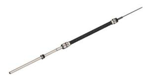
The model N9001 series RTD is designed for use as a wide range thermowell mounted sensor in the the primary coolant loop of PWR (Pressurized Water Reactor) nuclear generating facilities. The RTD is qualified per IEEE 323-1974/1983 and IEEE 344-1975/1987 for use in Class 1E harsh environments, but can also be used for non-safety applications.
