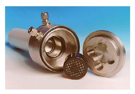
In operation, gas is pulled through the radioiodine collection cartridge by a vacuum pump. An in-line digital flow sensor measures the flow through the filter to ensure the optimum flow rate and to determine the air volume to be used in the calculations.
