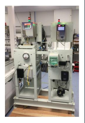
The SmartMCA uses Ethernet communications and is easily integrated into larger systems. It supports area monitoring (room air) applications as well as stack monitoring applications. Analog inputs for stack flow and outputs for system integration are standard. Bespoke stack flow and stack sampling systems are available from Ultra Energy.
